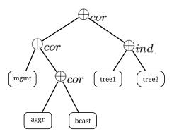
**Figure 2.** Composition hierarchy used in the third generation of the hypothetical example, showing management, aggregation, broadcast, and two spanning tree building sub-protocols.  $\oplus_{cor}$  is used for performance, and  $\oplus_{ind}$  is used to combine the two spanning-tree protocols to promote independent network overlays.
