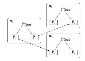
Figure 5. Independent merge: Sub-protocols on node  $n_1$  make independent peer selections and gossip separately. The merge operator increases its rate to keep each sub-protocol running at its requested speed.
